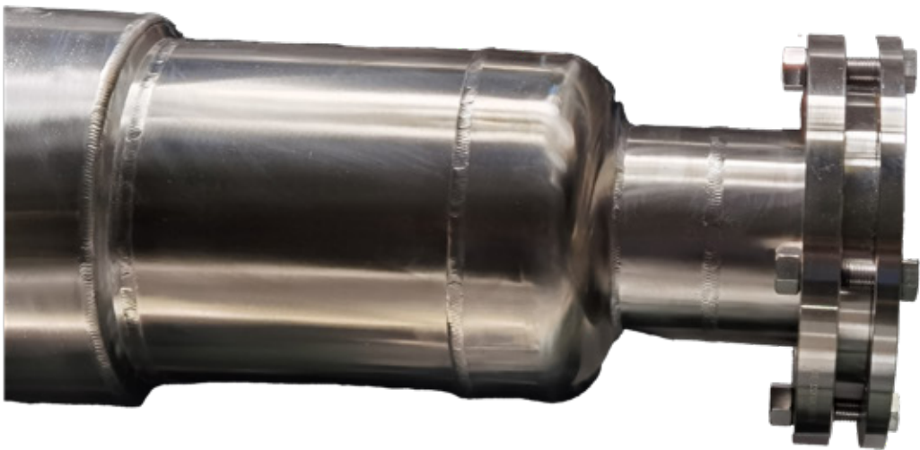
A FLANGE is re-welded on a welded coupling
